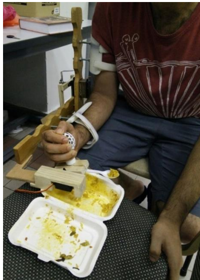
Figure 6. Forearm supination with the robot's assistance for eating
