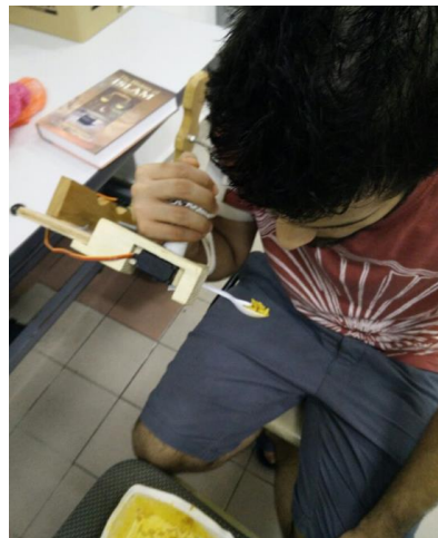
Figure 7. Elbow flexion with the robot's assistance for eating.
