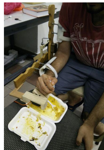
Figure 5. Forearm pronation with the robot's assistance for eating.
