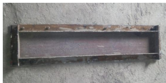
Figure No. 1. Sample Mould for Casting
