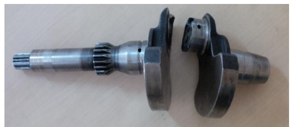
Fig. 1 Final failure On fillet of crankshaft
