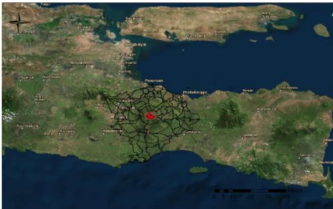
Figure 4. The estimation area which affected by lava flow based on interpretation of Mt. Bromo in the past eruption and simulation by using Lahar-Z application.
