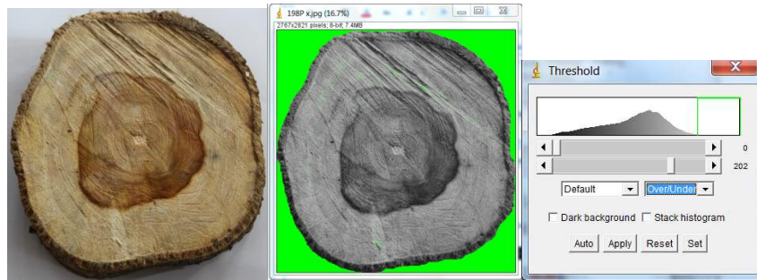
Figure 1. Automatic image processing procedure using ImageJ® to determine heartwood percentage from digital images of disk sections
