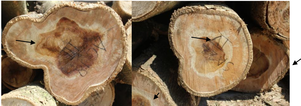
Figure 4. Transition zone (arrows) as it appears in cross sections of all logs cut from 5-year old fast grown teak trees
