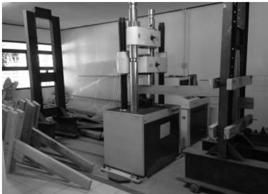
Figure 6. UTM and setup of the specimen.
