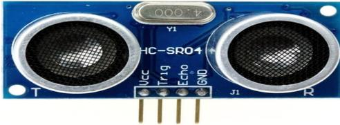
Gambar 1. Sensor Ultrasonik
