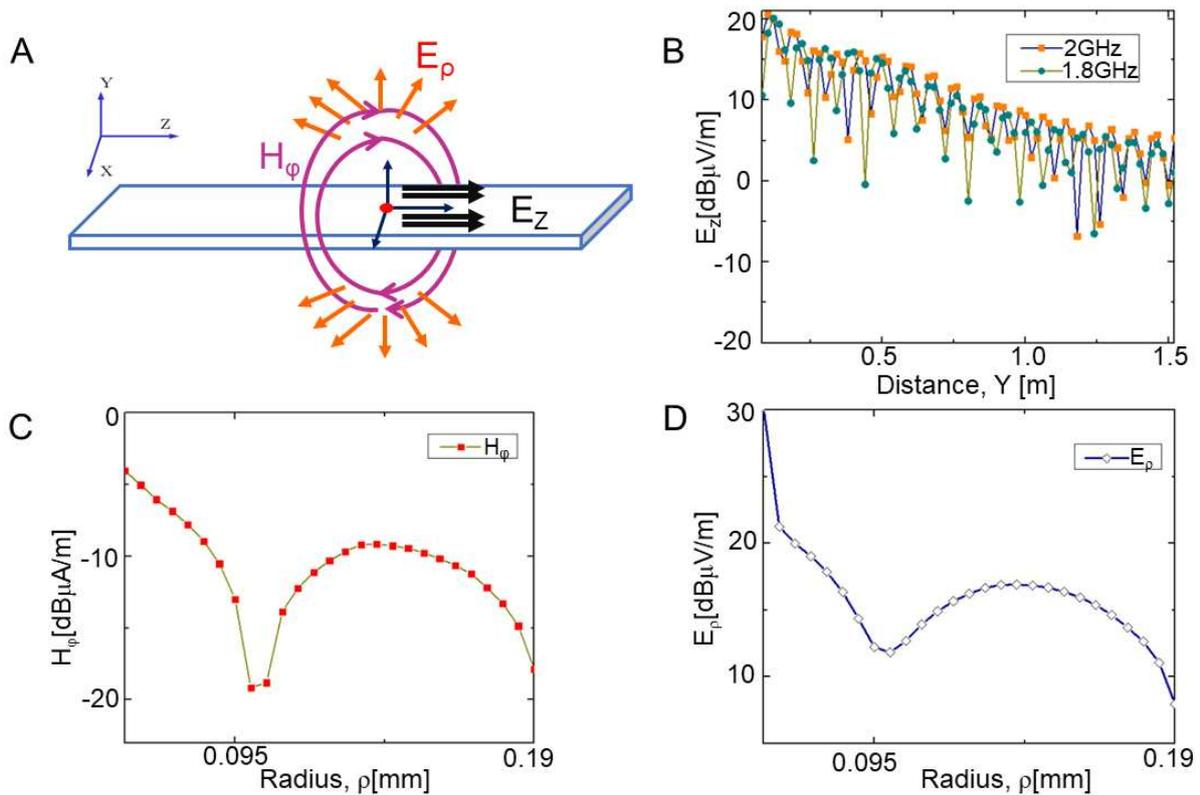
Figure.4. Field Profiles: A. TM Mode Fields around the metal due to excitation of Zenneck Waves; B. Electric field attenuation along the metal air interface independent of Frequency; C. Magnetic field radial decay away from metal; D. Electric field radial decay away from metal.
