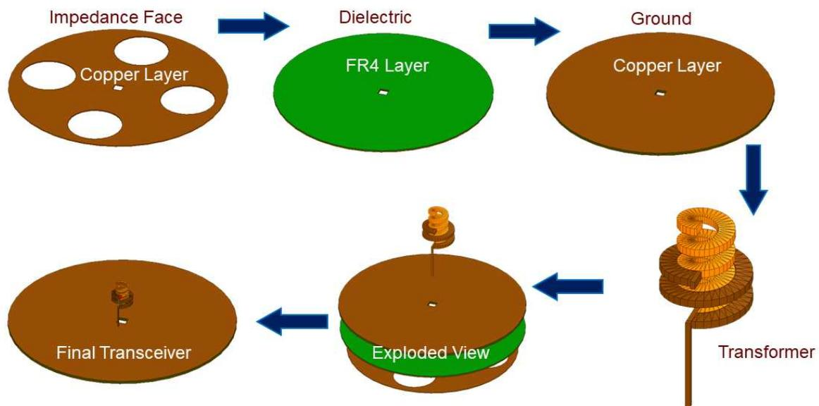
Figure.2. Prototype Fabrication steps and FEM Model; Excitation is provided across the transformer terminals
