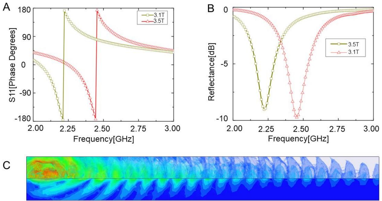
Figure.3. Simulations: A Reflectance in degrees. B. Reflectance in decibels C. E-field modes or Zenneck Iso-phase along a metal of 1540mm length.
