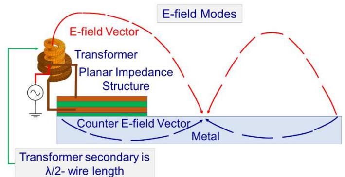
Figure.1. Concept Diagram: E-field modes generated by the resonator system on metal surface
