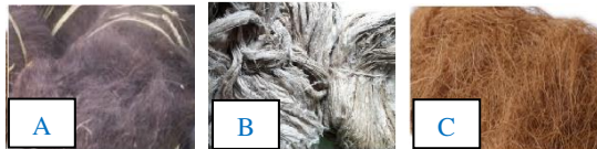
Gambar 2 Bahan baku serat hayati: (A) ijuk; (B) rami; (C) sabut kelapa.
