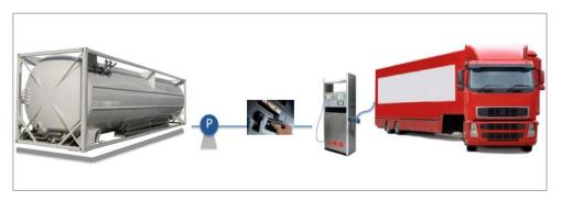
There are three options for LNG fueling: mobile containerized stations (20' or 40'), movable skidded stations and permanent full scale stations.
