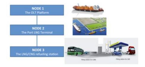
**NODE 1 - The OLT Platform**: FSRU Station - Floating Storage Regasification Unit, developed by OLT - Offshore LNG Toscana S.p.A. (OLT in the following) is one of the most important projects of national interest in the energy sector.
