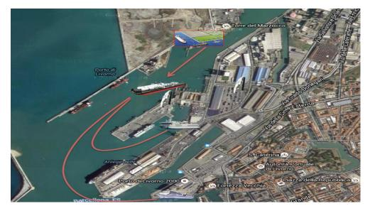
LNG Cryo-containers are taken from the Livorno port terminal (node 2), where they are stacked, loaded on barges best suited for port service to LNG powered ships berthed in the port; no specific manipulation must be done in the terminal, only a normal container loading operation made by a reach-stacker of the same type already present in the terminal.
