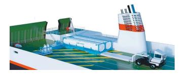
A fuel gas handling system utilizing removable LNG fuel tank containers is an option applicable to small and medium sized vessels, which do not require a large LNG capacity; such a solution offers a viable alternative to conventional stationary LNG tanks.
