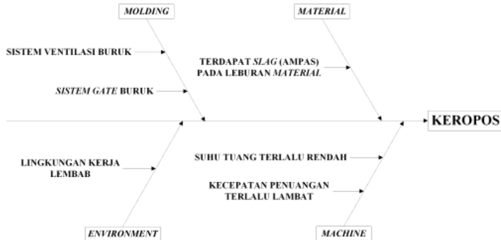
Gambar 4. Diagram Sebab Akibat ( Fishbone Diagram ) (Sumber: Pengolahan Data)
