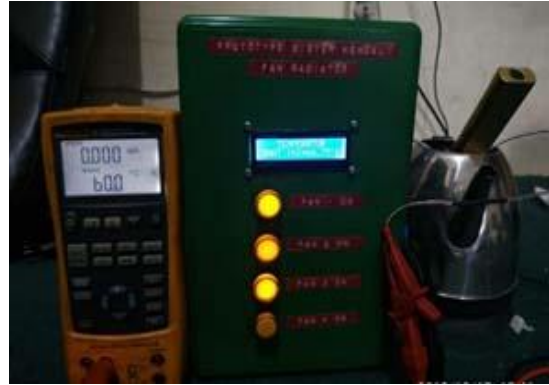
Picture 6. Fan Indicator Lights 3 Is On
