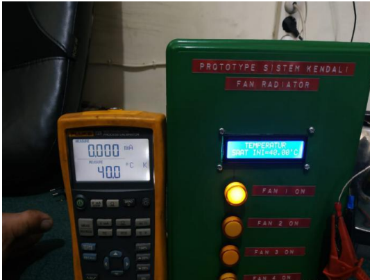
Picture 4. Fan Indicator Lights 1 Is On
