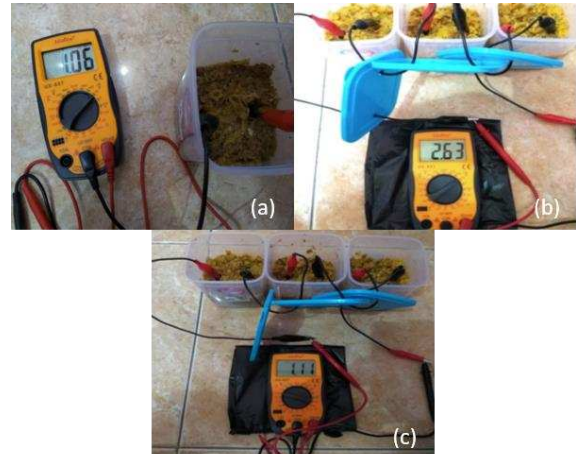
Figure 3. the voltage measurement (a) of SC and the voltage (b) and current (c) measurements in 3-SCs system, respectively.
