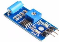
Gambar 3. Vibration Sensor
