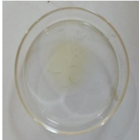
Figure 4 shows the disintegration of Films after being immersed in 0.1M NaOH for 5 days, it displayed that the Films, disregard of CNF Loading, are unstable at alkaline conditions.
