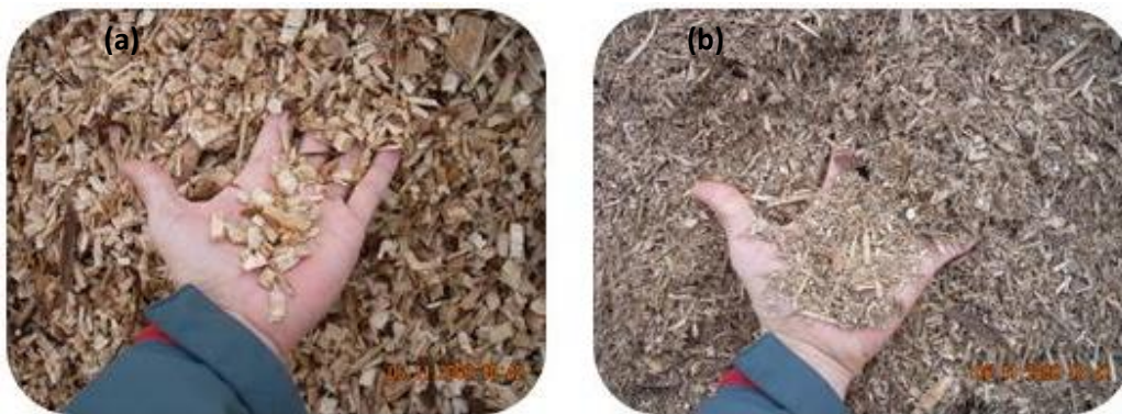
Figure 1. Wood residues tested as materials for the removal of nutrients from nutrient-rich effluents. G30 (a), 1-2 cm in length. Sawdust (b), 150 \mu\text{m} to 9.5 mm in length.
