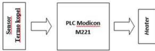
Gambar 1. Blok Diagram Kendali Suhu Oleh Sensor Termokopel
