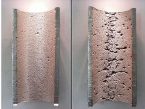
Gambar 2. Korosi Pada Pipa Boiler (Onny,2013)
