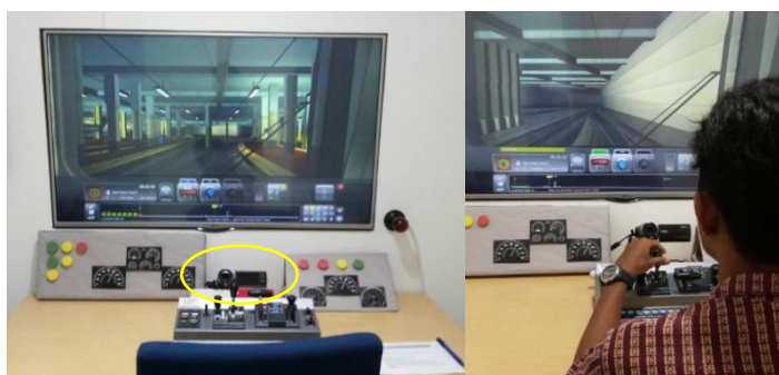
Gambar 1. Simulator Kereta Api di Laboratorium Fatigue
