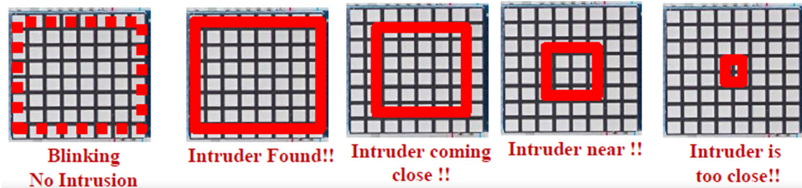
Figure 6. Four stages on 8x8 LED display
