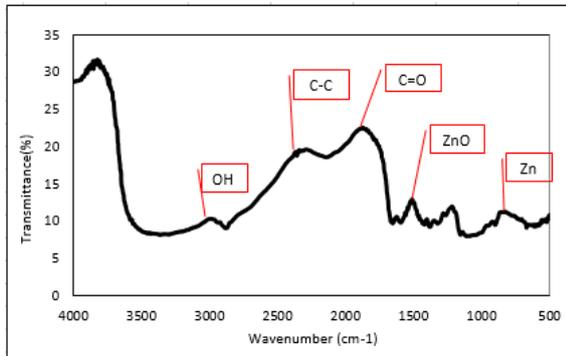
Gambar 3. Spectrum of FTIR ZnO Nanoparticle
