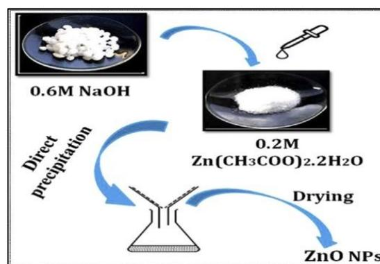
Gambar 1. Synthesis of ZnO Nanoparticles
