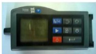
**Gambar 7.** Alat *Surface Roughness*
