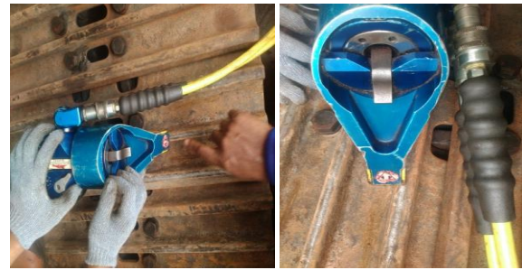
Gambar 4. Hydraulic Torque Wrench tanpa Holder
