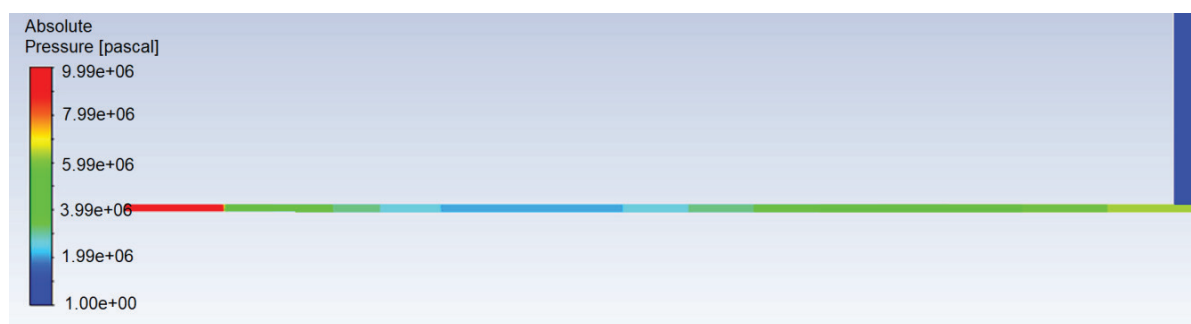
Fig. 3. Distribution of pressure fields along the unit barrel
