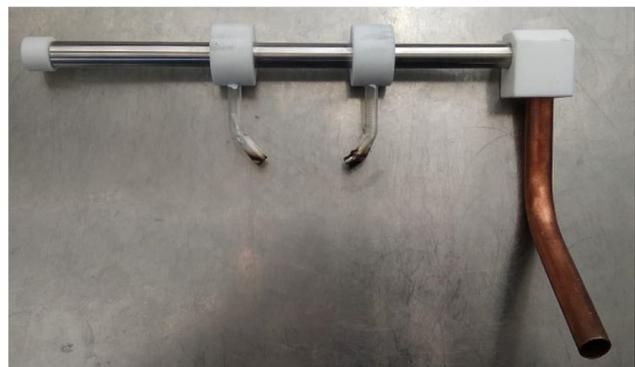
Fig. 9. Photograph of the gas-distributing tract used for the application of the coating on the piston
