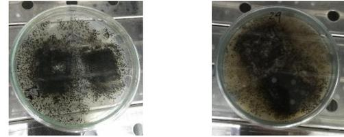
**Gambar 6.** Hasil biodegradasi H-14 bioplastik (a) 0% ZnO (b) 3% ZnO
