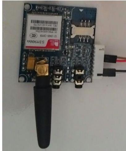
**Gambar 4.** Modul GSM SIM900A
