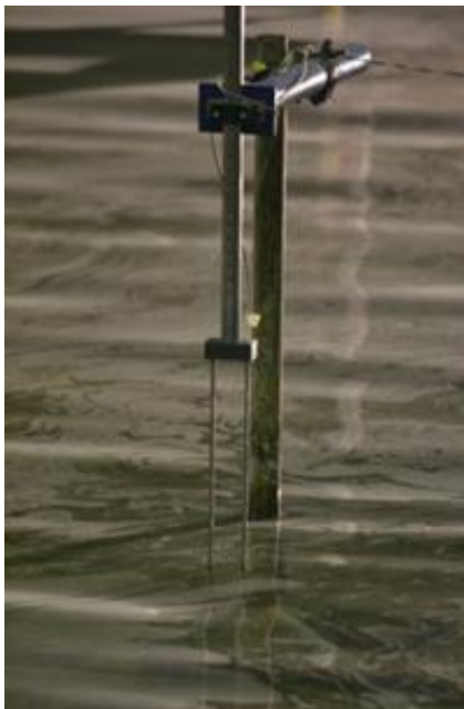
Gambar 11. Wave Height Sensor
