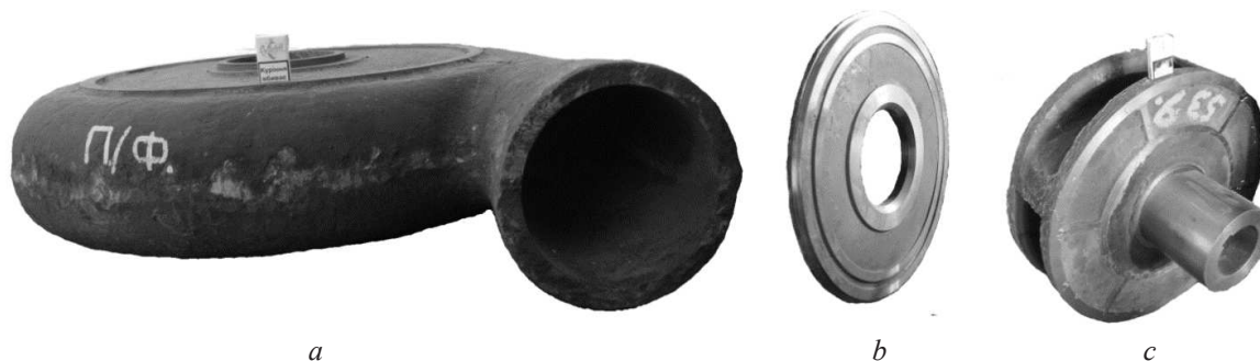
Fig. 6. Fast wearing parts of ash pumping systems of ash pumps at thermal power stations: a – a body, b – a disk, c – a wheel
