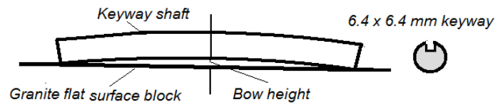
Fig. 4. Keyway shaft distortions [6]
