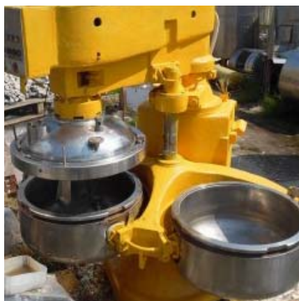
Fig. 1. Cooper of melting cheese V2-OPN 1200 kg/hour
