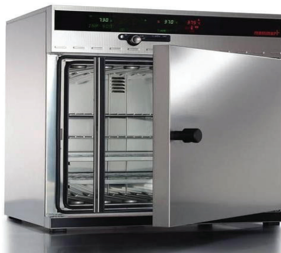
Fig. 1. Thermostat by Memmert IPP-200 (Germany)
