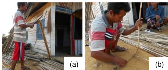
Figure 4. (a) The process of splitting bamboo wood and (b) The process of slicing bamboo fragments.
