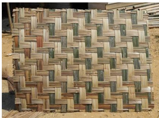
Figure 6. Material of woven bamboo walls that have been finished.
