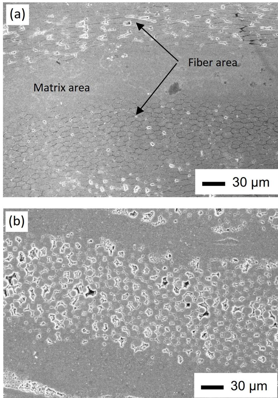
Figure 1. SEM Images of SiC<sub>f</sub>/SiC composites: (a) nSiC and (b) pSiC
