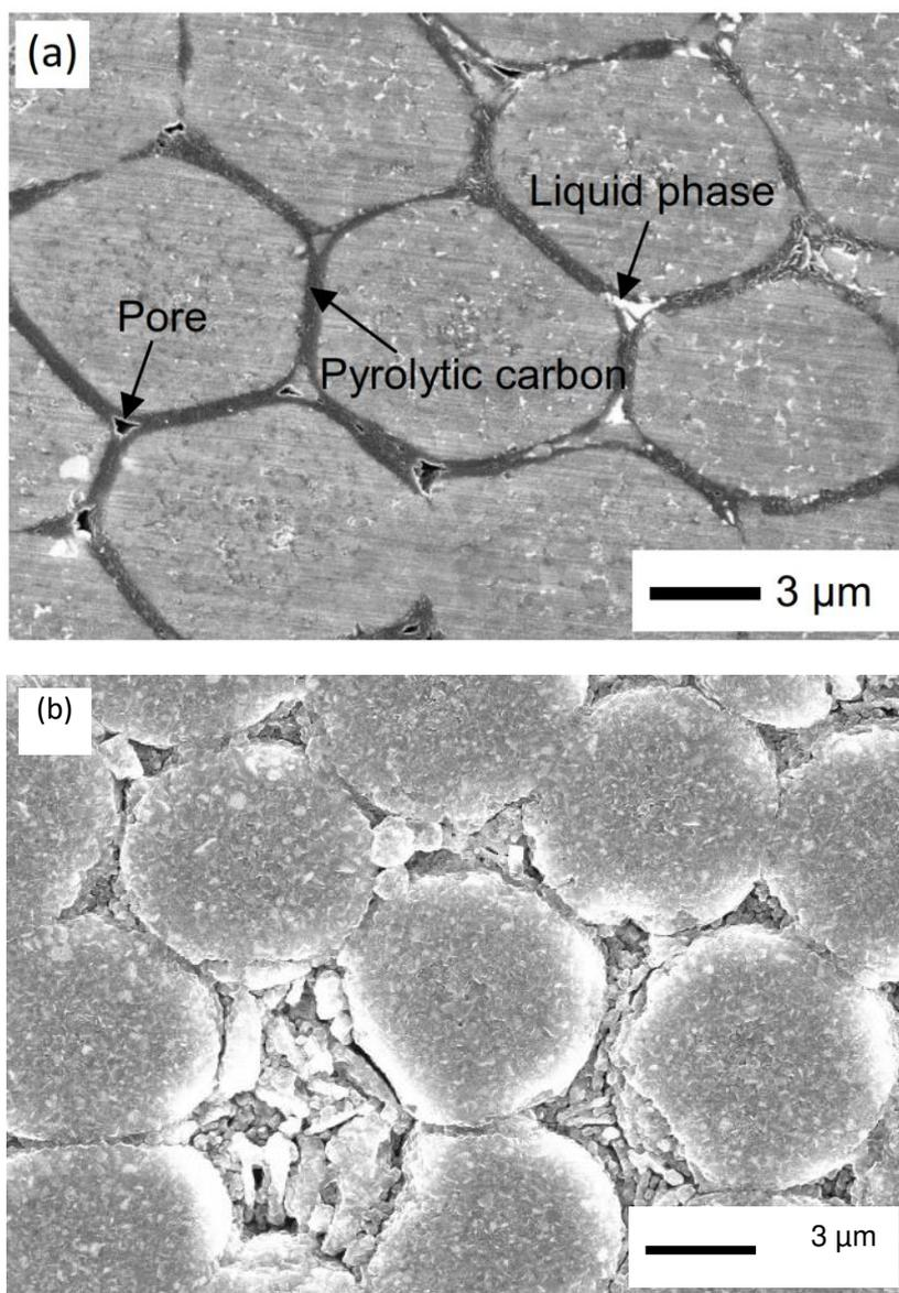
Figure 2. SEM Images of fiber area in the SiC<sub>i</sub>/SiC composites (a) nSiC and (b) pSiC
