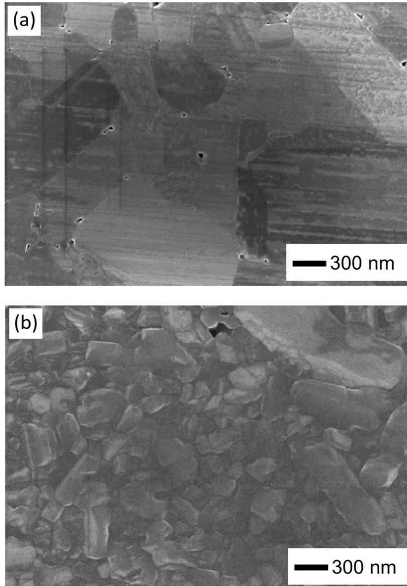
Figure 3. SEM Images of grain size in the matrix area of the SiC<sub>i</sub>/SiC composites (a) nSiC and (b) pSiC
