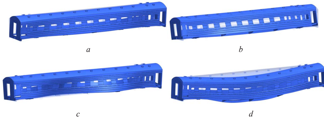
Fig. 9. Forms of oscillations of the body of a passenger car when transported by rail ferry: a – the first form; b – the second form; c – the third form; d – the fourth form
