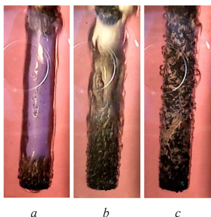
Fig. 4. Film boiling a and creation of insulating surface layer b during quenching of cylindrical probe 12.5 mm in diameter in mineral oil I-20A which were captured by video camera: a – film boiling at the moment 1.5 sec when core temperature is 780 °C; b – film boiling is almost finished at the moment 3.2 sec when core temperature is 720 °C and formation of insulating layer starts; c – nucleate boiling process on the surface of insulating layer during cooling in oil I-20A at 50 °C at the moment 5.8 sec when core temperature is 525 °C
