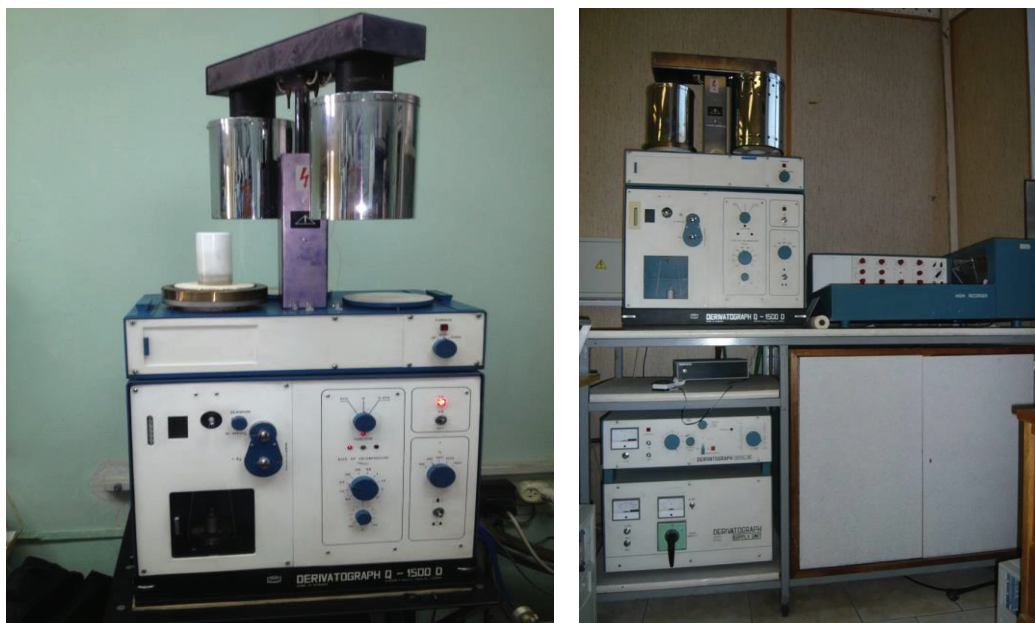
Fig. 2. Visualization of the measuring laboratory device derivatograph Q-1500 D
