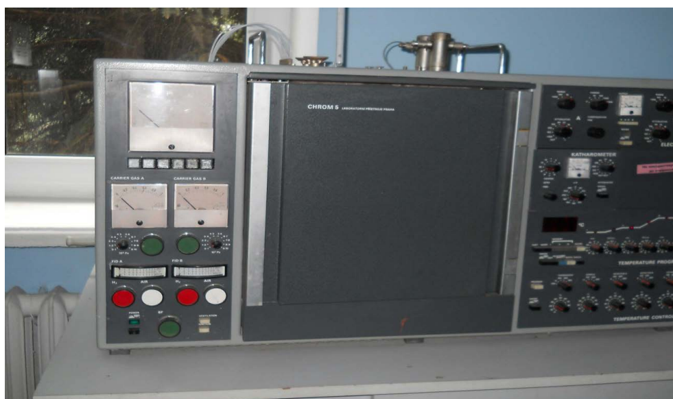
Fig. 3. Device chromatograph “Chrome-5» for determination of fatty-acid composition of the control and development batches of sour cottage cheese of goat milk (USA)
