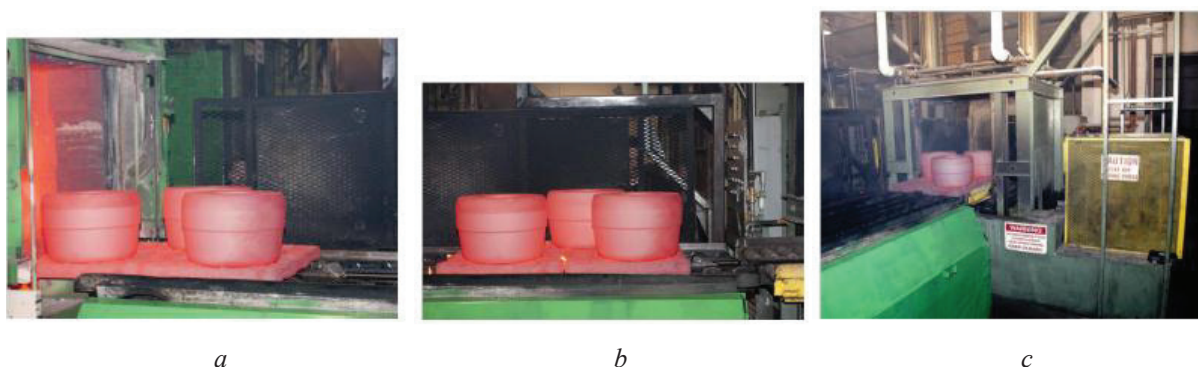
Fig. 1. Standalone 23 m 3 IQ water tank installed across atmosphere box furnace at Akron Steel Treating Co. [7, 8]: a – load is exiting the furnace; b – load is on the transfer cart; c – load is entering the IQ tank
