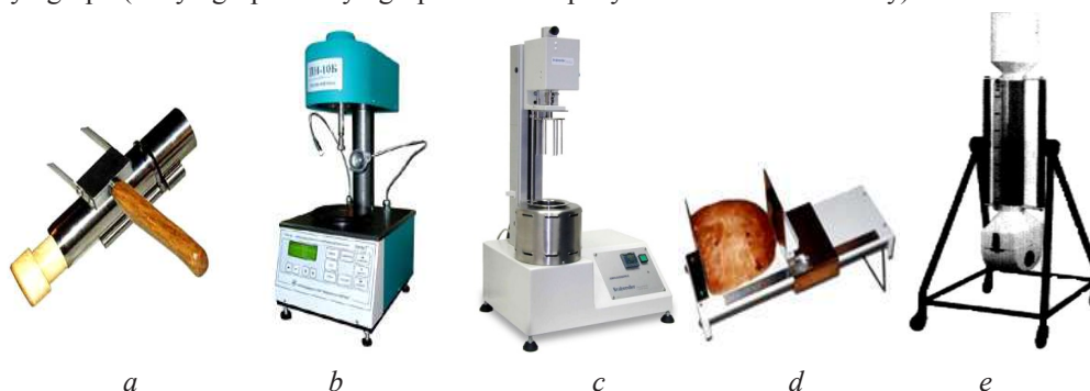
Fig. 2. Devices used for research of qualitative indicators of bread: a – device Zhuravlev; b – penetrometer AP-4/2; c – amylograph-E; d – VFH-250; e – volume RZ-BIO
