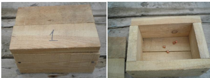
Fig. 1. Untreated model sample of the containers for storage of ammunition
