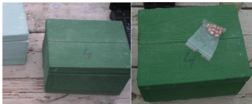
Fig. 4. Fire resistant model sample of the containers for storage of ammunition, which is treated with geocement coating with heat-reflecting screen
