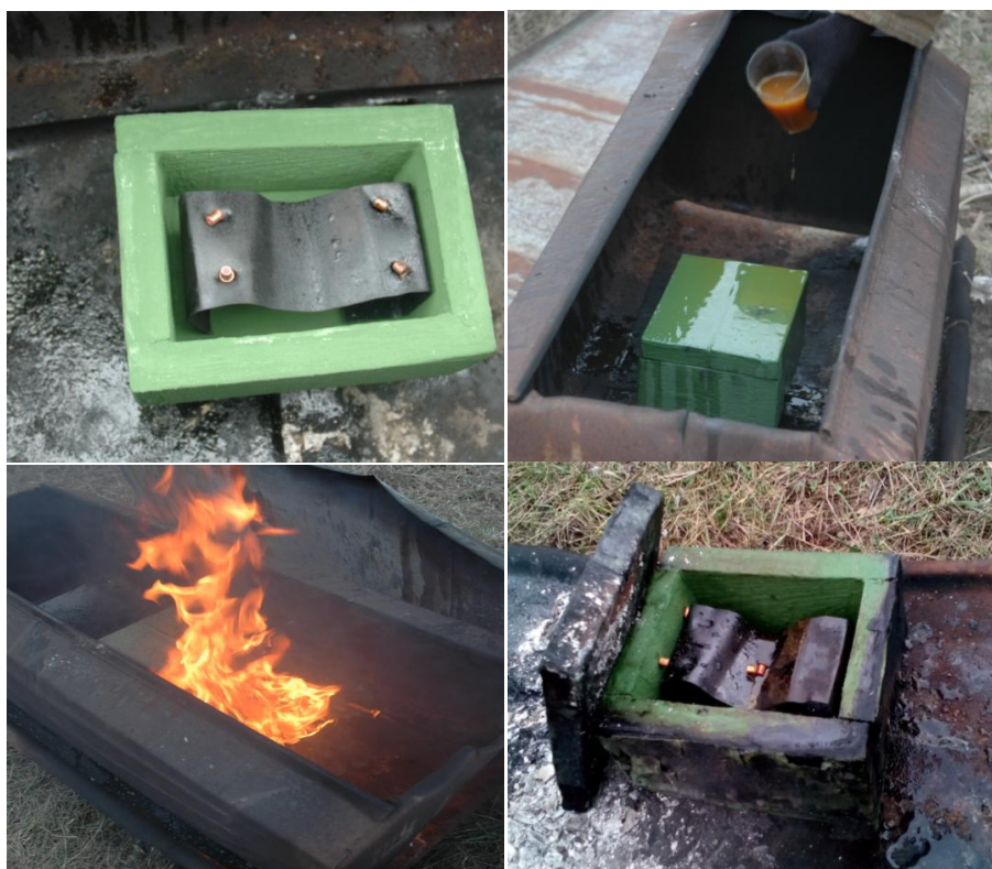
Fig. 12. Fire test results for model sample of the containers for storage of weapons and ammunition treated with geocement coating with heat-reflecting screen
