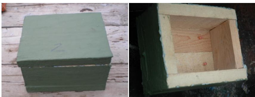
Fig. 2. Fire resistant model sample of the containers for storage of ammunition, which is treated with a fire retardant coating (utility model patent of Ukraine № 95440)
