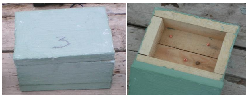
Fig. 3. Fire resistant model sample of the containers for storage of ammunition, which is treated with organic-mineral fire retardant coating
