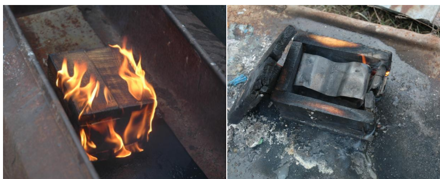
Fig. 6. Fire test results for untreated model sample of the containers for storage of weapons and ammunition
