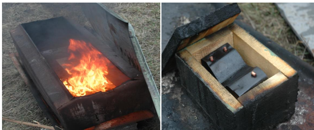
Fig. 10. Fire test results for model sample of the containers for storage of weapons and ammunition treated with organic-mineral protective coating
