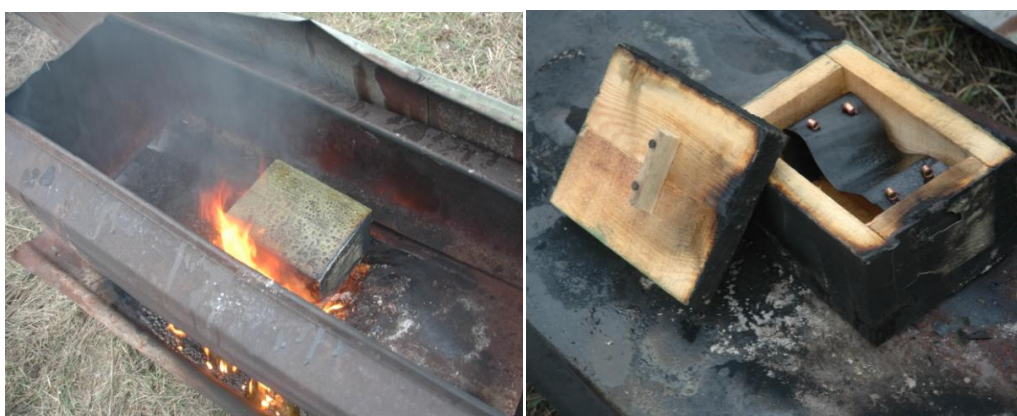
Fig. 8. Fire test results of model sample of the containers for storage of weapons and ammunition treated with fire retardant coating (utility model patent of Ukraine № 95440)
