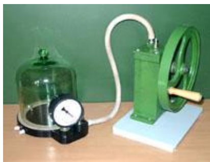
Fig. 14. Kamovsky electrovacuum pump with dilution 13 Pa
