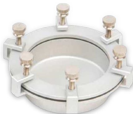
Fig. 2. Dish for measuring steam permeability
