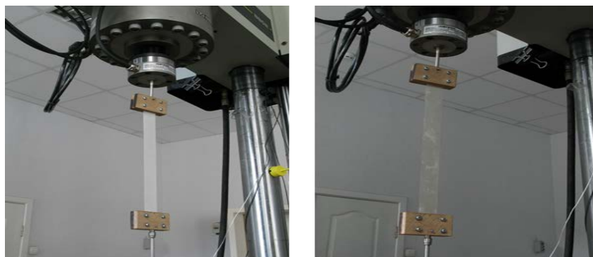
Fig. 3. The study of mechanical characteristics of the film-forming coat
