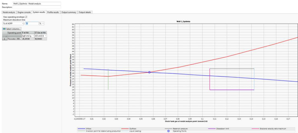
Fig. 6. Graph of inflow-outflow of well fluid of Opishnia oil and gas condensate field (Well No. 1) (base)
