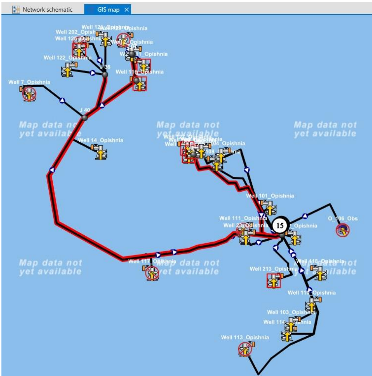
Fig. 3. The gas gathering system of the Opishnia OCGF
