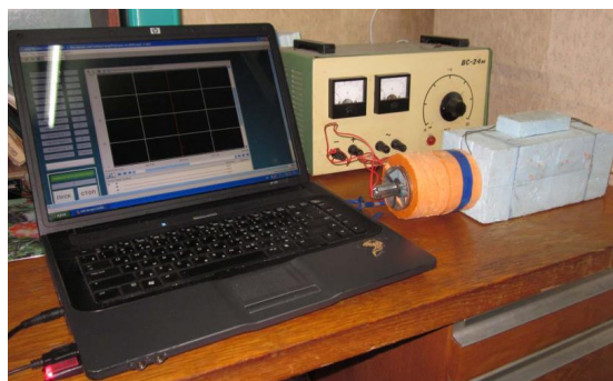
Fig. 1. Laboratory low-temperature calorimeter with analogous-digital transformers, produced by DCON Utility (USA)
