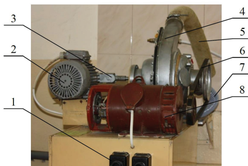
Fig. 3. General view of the experimental setup of PM with VR: 1 – control stand; 2 – electric motor of rotor vibration drive; 3 – crank gear; 4 – homogenizing unit; 5 – branch pipe of the product discharge; 6 – cone belt transmission of rotation of rotor; 7 – branch pipe of milk supply; 8 – electric motor of the rotor rotation drive
