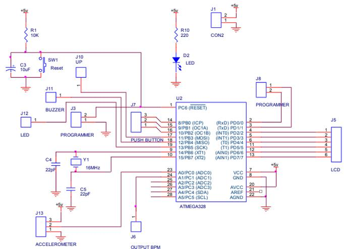
Fig. 3. Minimum System Arduino ATmega 328
