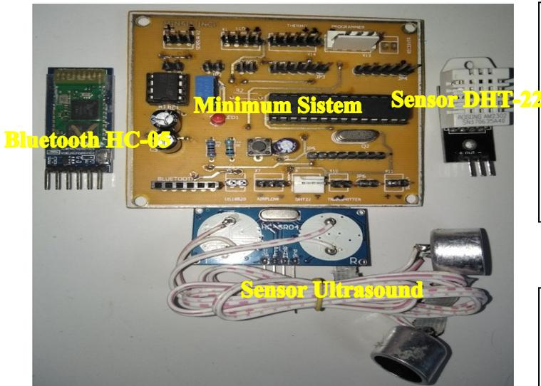
Fig. 9. The Digital part of the Incubator Analyzer
