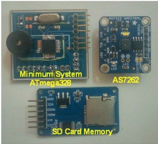
Fig. 5. The digital part of the phototherapy radiometer
