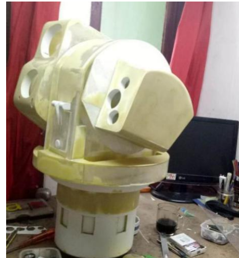
Figure 4. Putty process (Source: Hardy Adiluhung 2018)
